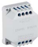
Relay for Blinds Control - Rated voltage: 230V~ – 50Hz. - Breaking capacity: 6A. - Not temporized. - Connect locally to Venetian Double Push-button (Ref. 21283) - For the centralized command of the installation, connect remotely to a Venetian Double Push-button (Ref. 21283) • See Technical Data Sheet - page 40
