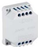
Automatic Relay for Blinds Control - Rated voltage: 230V~ – 50Hz. - Breaking capacity: 6A. - Temporized. - Connect to the Double Push-buttons and to the Venetian Double Push-buttons. • See Technical Data Sheet - page 39
