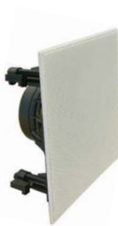
Squared Grid 2-Way Loudspeaker of 6,5" - 32 Ohm - External dimensions (mm): 220 x 220 x 93. - Maximum power: 60W. - Frequency response: 60 - 20000Hz.
