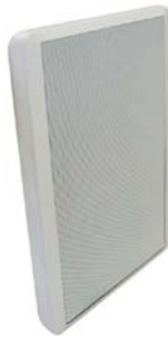
Surface Mounting Flat 2-Way Loudspeaker of 5" - 32 Ohm - External dimensions (mm): 274 x 185 x 36,5. - Maximum power: 15W. - Frequency response: 80 - 19000Hz.
